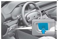
1. Press and hold the tailgate open button located on the instrument panel to open the power tailgate.
