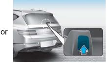
1. Press the tailgate open button located outside the tailgate while carrying the smart key to open the power tailgate.
