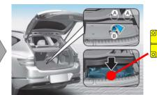
2. To access the battery, remove the clip (A) and release the cover (B).
