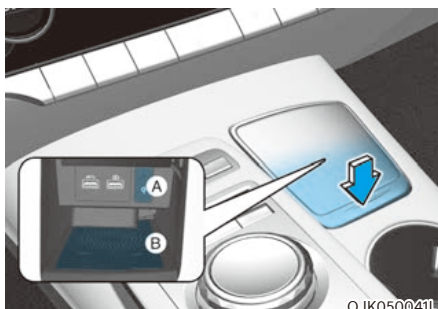
[A] : Indicator light, [B] : Charging pad
