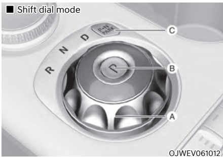
[A]: Rotary shifter(Rotary gear shift dial), [B]: P button, [C]: P release cap
