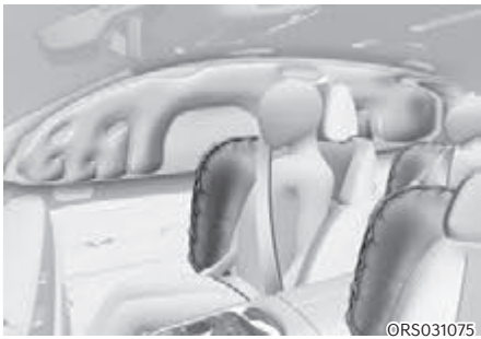
[A]: Side air bag(Front row), [B]: Side air bag(Second row), [C]: front center side air bag (Driver's seat)
