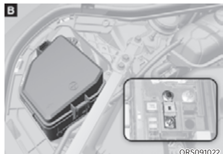
[A]: Multi type fuse, [B]: Midi type fuse
