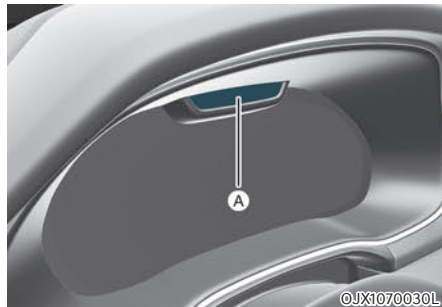
[A] : Interior view camera
