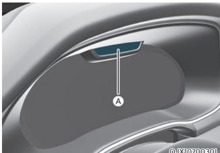
[A]: Interior view camera
