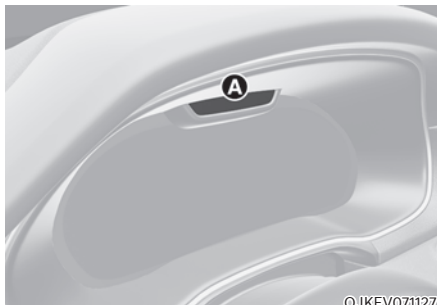
[A]: Interior view camera
