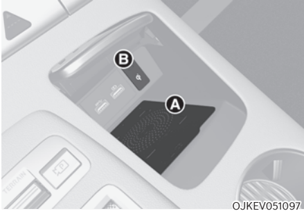
[A]: Charging pad, [B]: Indicator light
