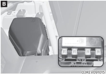
[A]: Blade type fuse, [B]: Cartridge type fuse
