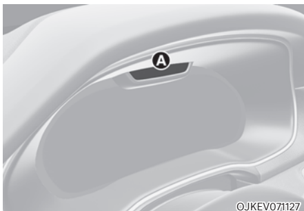
[A] : Interior view camera
