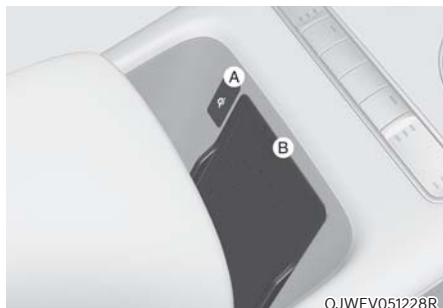
[A] : Indicator light, [B] : Charging pad
