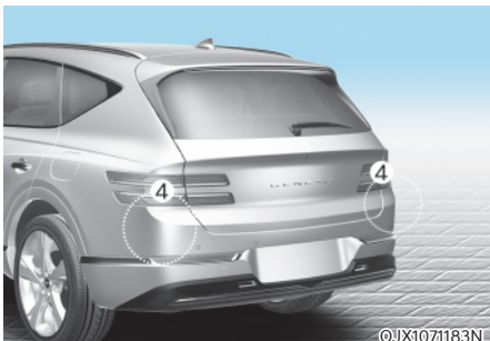
[1] : Front view camera, [2] : Front radar, [3] : Front corner radar (if equipped), [4] : Rear corner radar (if equipped)
