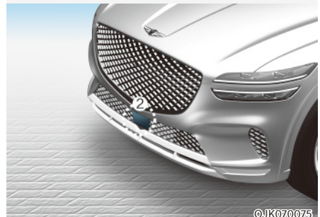
[1]: Front view camera, [2]: Front radar
