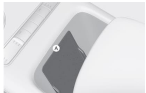
Ⓐ: Put your device on this charging pad
