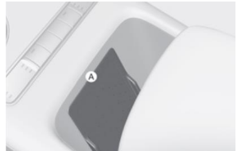
Ⓐ: Put your device on this charging pad
